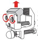
Re-tighten screws and fully engage the lock washers.
