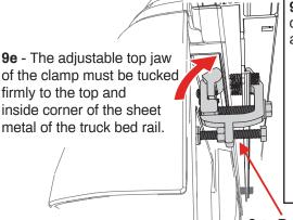
**9f** - If the jaw does not contact firmly into the corner of the bed flange, remove the clamp and loosen the screws to adjust the jaw.
