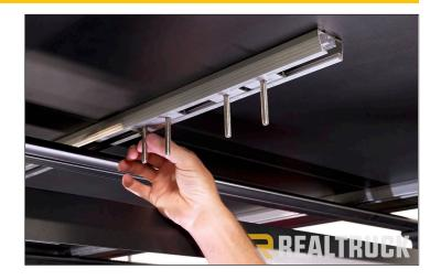
8. Place the Large Bolt Plate (#7) under your crossbar and into each bolt. There are two hole options on the large bolt plate to allow you the best fitment in your application. Use the M8 Locking Nuts (#10) to the bolts. DO NOT over tighten this hardware! Over tightening could bend the bolt plate or crush your crossbar. Secure all 4 mounting locations and fully tighten.
