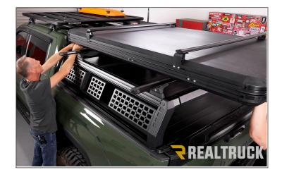
6. Pull the plastic cap off the end of the aluminum track on the bottom of the GoTent. Place a M8 Hex Head Bolt (#9) into the Small Bolt Plate (#6), then slide the Small Bolt Plate (#6) into the track. Insert 4 per track. Reinstall the plastic cap to the end of the aluminum track. Repeat on the other track.
