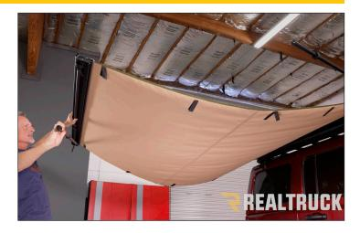
11. While holding the awning end beam with one arm, slide out each rafter arm, aligning the end pin into the end beam holes, then twist the arm to lock in position. Fix the awning fabric to the rafter arms using the Velcro straps.
