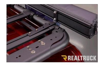
6. Tighten the hardware attaching the Mount Bracket (#2 or #3) to your storage system. Now, tighten the hardware attaching the Mount Bracket (#2 or #3) to the Roof Top Awning (#1).
