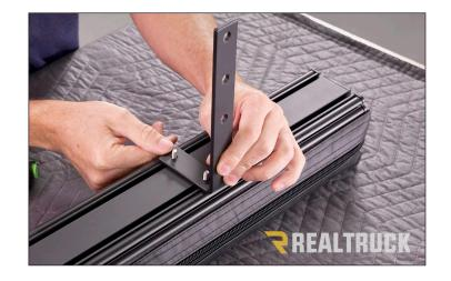
3. Measure to the desired mounting location on the roof rack. Move the brackets to that position. Place M6 Flat Washer (#8) and M6 Locking Nut (#9) to the bolts and loosely tighten.
