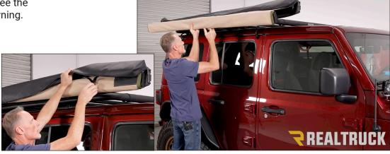
9. While holding the awning, gently swing out both awning rafter arms slightly past 90 degrees away from the vehicle allowing the awning to roll out between them.
