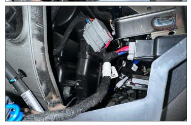
14. From underneath the cab, feed the extension harness through the rubber grommet under the driver's side carpet.
