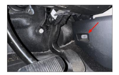
17. On the passenger kick panel, remove the fuse block cover. Using the fuse plug on the provided extenion harness, remove the 5 amp fuse in slot 30. Plug this fuse into the provided fuse plug harness if fuse is not preinstalled.
