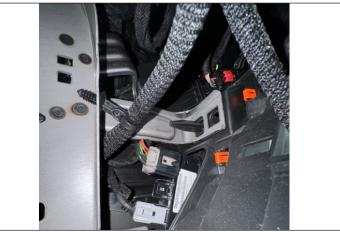
14. Plug the 4-pin plug into the T-harness.
