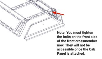
5. Install the 2 Top Support Members (#6) to the top of the rack using 4 M8 x 1.25 x 20mm Bolts (#10) and 4 M8 Washers (#11) on each support member. Loosely fasten.
