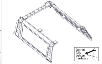
3. Working your way toward the rear/tailgate, install Crossmember, Middle (#4) to Side Panel, Driver Side (#1) from Step 1 and Side Panel, Passenger Side (#2) with 2 M8 x 1.25 x 20mm Bolts (#10) and 2 M8 Washers (#11). Loosely fasten.
