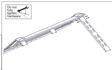
2. Install Side Panel, Passenger Side (#2) to Crossmember, Cab End from Step 1 with 2 M8 x 1.25 x 20mm Bolts (#10) and 2 M8 Washers (#11). Loosely Fasten.
