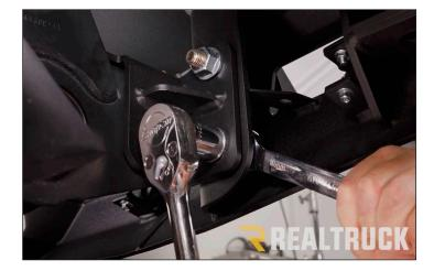
**STEP 18:** Adjust the frame mount to side protection to ensure that the hardware is not binding. Then, fully tighten the frame mount to the frame.
