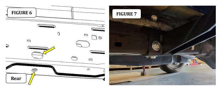
**Step-6** Align the Frame mount slider with the vehicle and tighten all bolts and nuts securing the slider to the front, center and rear brackets. Repeat the above steps to install the passenger side Frame mount slider. Remember to check and retighten the nuts every six months.
